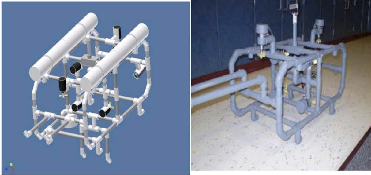
Figure 6. CAD depiction (left) and an “Almost Final” photograph (right) of the ROV designed and constructed for the MATE competition by the HSE team from Utica Community Schools, Utica, MI.
