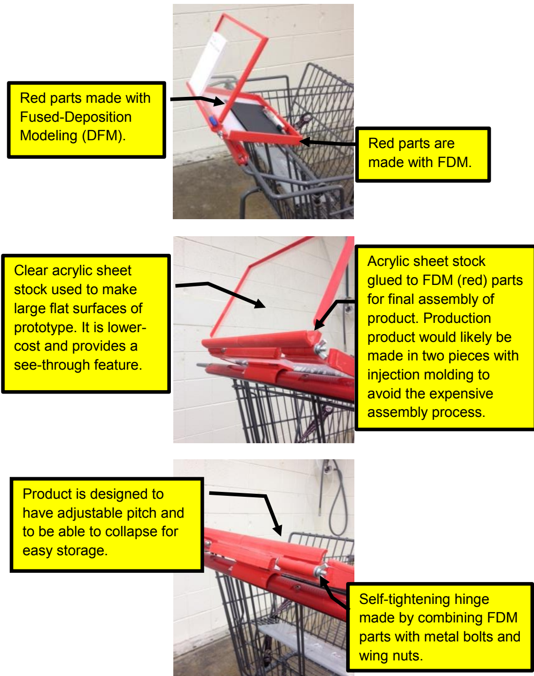
Figure 7. Alpha prototype: a high-fidelity prototype made primarily from FDM. Note the alpha prototype consists of FDM parts (red) and other plastics (clear panels of 1/8 inch thick acrylic sheet) and metal screws (self-tightening hinge). Acrylic is glued to the FDM plastic.
