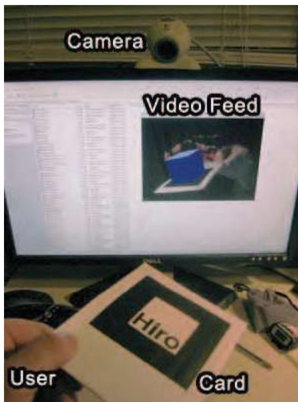
Figure 2. Monitor-Camera Augmented Reality Setup
