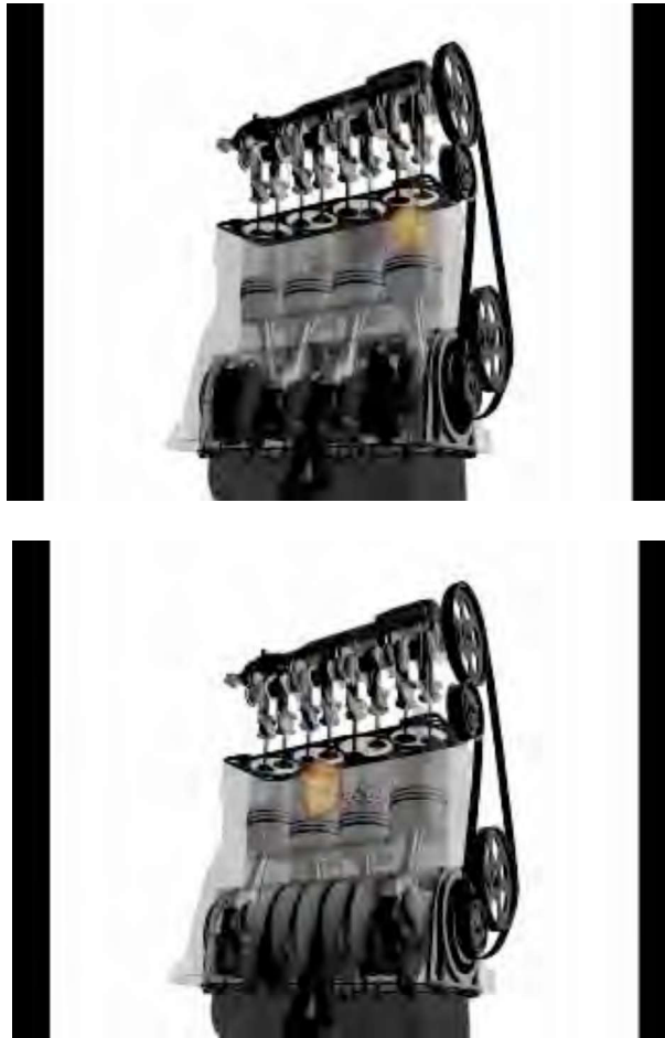
Figure 5. Two frames from the animation of a 4-cylinder engine, showing a simulation of the combustion process.
