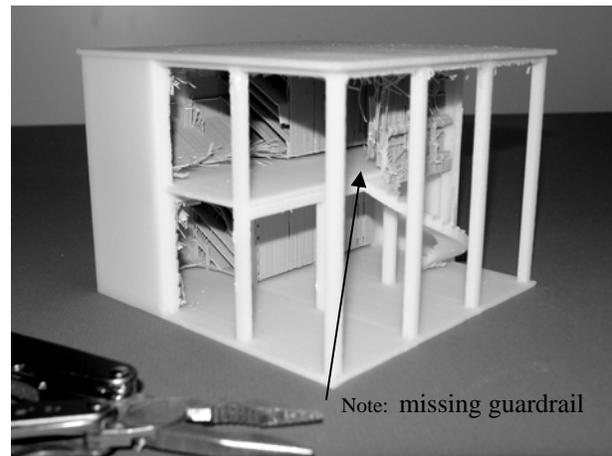
**Figure 4. Completed model after partial support material removal**
