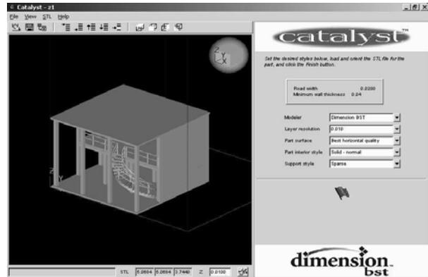
**Figure 3. Stratsys processing the model**
