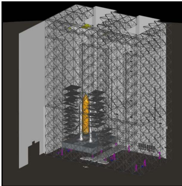
**Figure 1. VAB As A Simplified Rep (Including Structural Steel, Major, and Extensible Platforms).**
