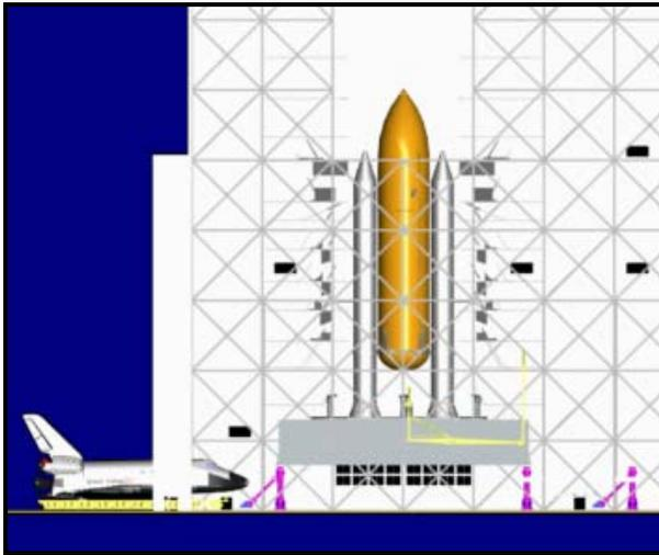
**Figure 3. Orbiter And Transporter (OTS) Entering VAB.**
