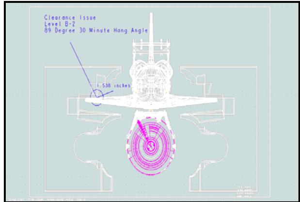
**Figure 8. Drawing Showing Clearance at B-2.**
