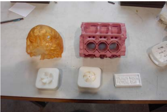
Figure 2: Some Examples of Parts created with Additive Methods
